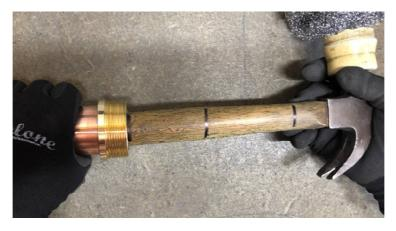
8. **Place the 5<sup>th</sup> piece of mesh into position** – and using only your fingers push it into the column so that the brass end piece is nearly all visible on the inside of the column. Cut off any loose strands.
