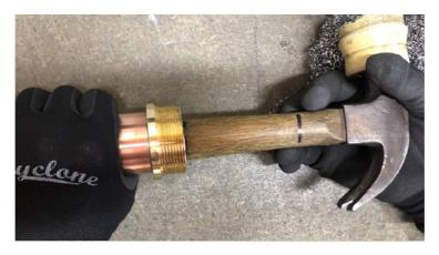
3. **Slide 3<sup>rd</sup> piece of mesh into position** – as per the previous pieces and use the hammer handle to gently tamper the mesh to the 7.5cm measurement. This will be considerably easier than the previous pieces.
