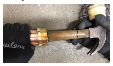
7. **Slide 4<sup>th</sup> piece of mesh into position** – as per the previous pieces and use the hammer handle to gently tamper the mesh to the 7.5cm measurement. This will be considerably easier than the previous pieces.
