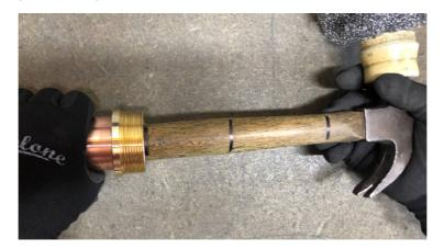
4. **Place the 4<sup>th</sup> piece of mesh into position** – and using only your fingers push it into the column so that the brass end piece is nearly all visible on the inside of the column. If you can't fit the 4th piece in comfortably, then cut it to size with scissors and fit as per photo below and cut off any loose strands.
