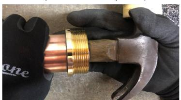
6. **Slide 3<sup>rd</sup> piece of mesh into position** – as per the previous pieces and use the hammer handle to tamper the mesh to the 15.0cm measurement. This will be considerably easier than the 2<sup>nd</sup> piece, if it isn't, remove all the mesh, gently fluff the mesh to its original form and start again.
