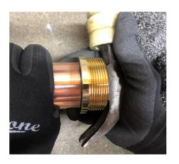
hammer length will slide in to the hammer head. There is no force applied in this step as we do not want to damage the thermowell.
